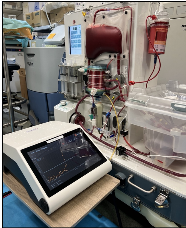
Figure 1: The LiMAX FLIP ® 4.0 detection device connected to the CO 2 outlet of the OrganOx metra oxygenator to allow quantification of the ^{13}\text{CO}_2 : ^{12}\text{CO}_2 ratio.
